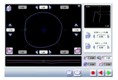
By default, the edger shows the values corresponding to the frame material (metal or plastic). Check and modify these values according to the thickness of your lens and your frame.
