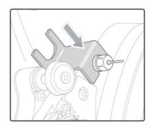
2 Put the adjustable wrench on the chuck
