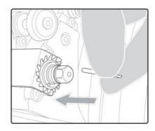
Put the adjustable wrench onto the chuck, then tighten (two notches towards the bottom of the trough).
