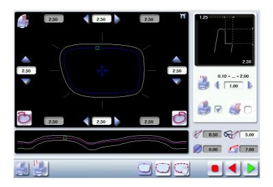
Press the buttons  $\overline{\langle}$  and  $\overline{\rangle}$  on the right of your screen to modify the width of the flat side of the bevel.
