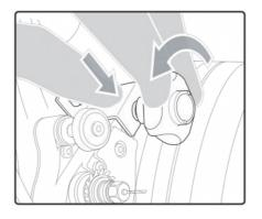
4 Remove the adjustable wrench then the drill bit.
