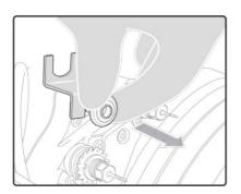
7 Position the "step ++" wheel on the axis.
