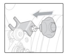
3 Loosen the chuck with the adjustable wrench (two notches towards yourself).
