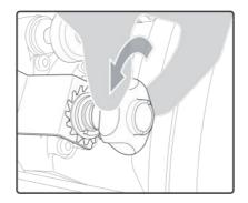
5 Remove the adjustable wrench then the mill bit.
