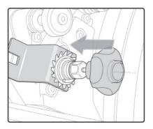
4 Loosen the chuck with the adjustable wrench (two notches towards yourself).
