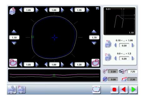
Press the buttons 🧹 and 🝺 on the right of your screen to modify the width of the flat side of the bevel.
