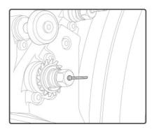
> The mill bit is in place.
