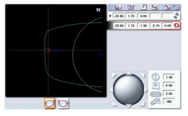
1 Press on the drill-hole, slot or notch to select it.
