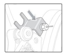
4 Put the adjustable wrench onto the chuck.
