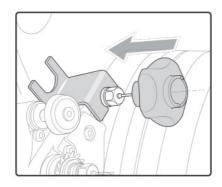
5 Loosen the chuck with the adjustable wrench (two notches towards yourself).
