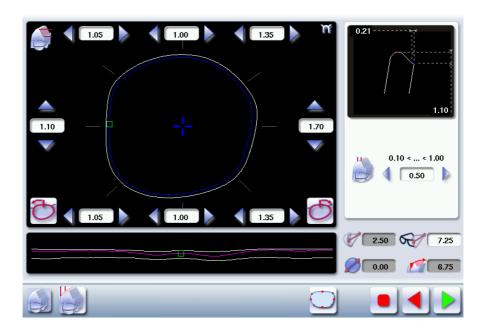
By default, the edger shows the values corresponding to the frame material (metal or plastic). Check and modify these values according to the thickness of your lens and your frame.
