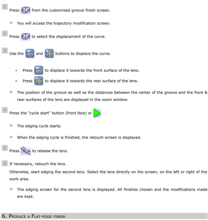
For a flat-edge finish, only automatic mode **equal** is accessible.
