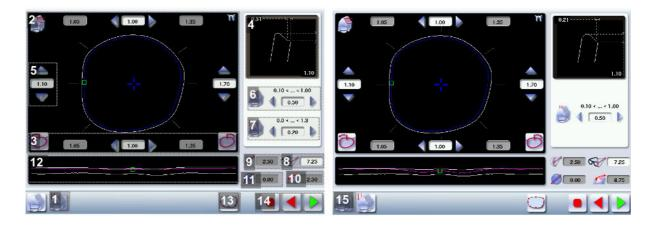
1. High-base bevel screen "front surface monitoring"
