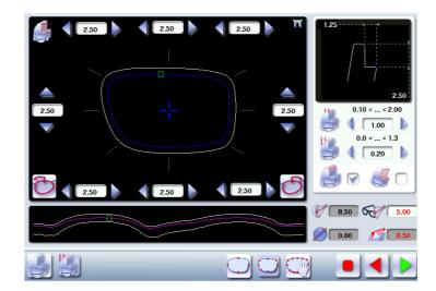
Press the  $\longrightarrow$  and  $\checkmark$  buttons to modify the shelf bevel value at each point of the shape in
