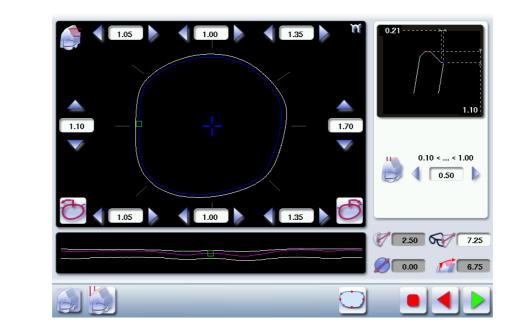
Press the buttons < and 📄 on the right of your screen to modify the width of the flat side of the bevel.
