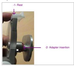
Make sure to align the horizontal of your pattern (or demonstration lens) and that of the pattern holder.
