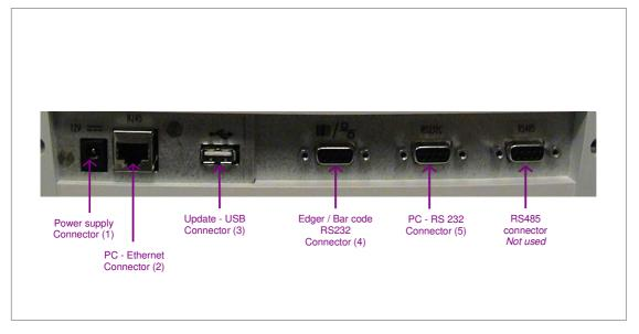
Depending on your configuration, your Essilor e-Tess tracer can be connected to either a PC or an Essilor Delta T edger.
