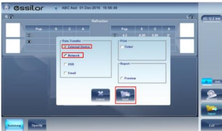
Select "External Device". Data are automatically transferred to essibox.com and available for APH550
