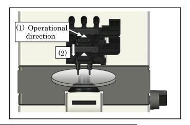
Do not give strong impact to a lens when lowering the lens holder. When rising the lens holder, make sure to move to the top.
