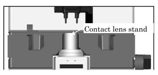
(3) Lower the lens holder, and hold the contact lens stand which the contact lens is already placed.
