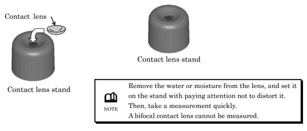
(2) Replace the standard lens stand with the contact lens stand.
