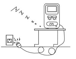
(5) Never attempt to fix or remodel the device. When the device fails to function properly, do not touch the inside. Contact us or your local distributor.
