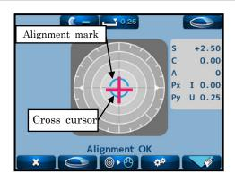
The alignment mark represents the optical center of the lensmeter and the cross cursor represents the optical center of the lens.
