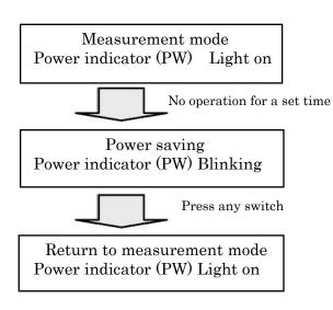
While this function is activated, the power to the measurement light and LCD monitor is turned off.
