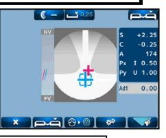
When "ADD Measure" on the Setup screen is set as "F/N.AT", it is detected automatically and the measurement values are stored in memory.
