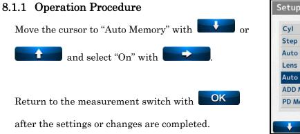
he measurement values are stored in memory automatically when the message "Marking OK" appears after the alignment mark and cross cursor overlap as shown on the right.
