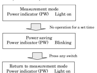
While this function is activated, the power to the measurement light and LCD monitor is turned off.
