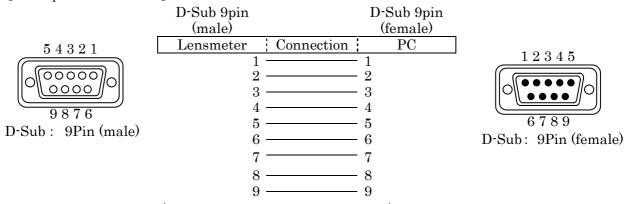
Use the straight cable (D-sub 9 pin: male/ D-sub 9: female) as the connection cable at the time of outputting the measurement values by using the RS232C.
