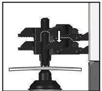
(4) The marking lever returns to the initial position.
