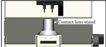
(3) Lower the lens holder, and hold the contact lens stand which the contact lens is already placed.
