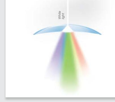
The ALM 500 and ALM 700 use a green light beam\* that reduces measurement drift due to light deviation by the lens.
